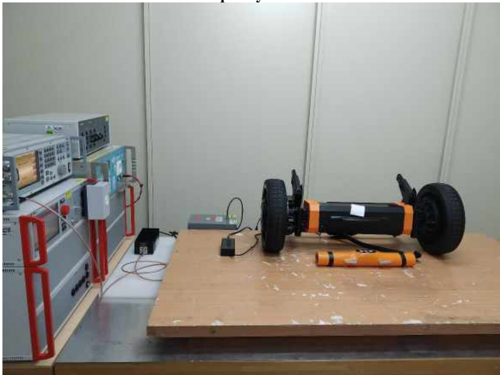
Picture 9: Continuous Induced Radio-Frequency Disturbance
