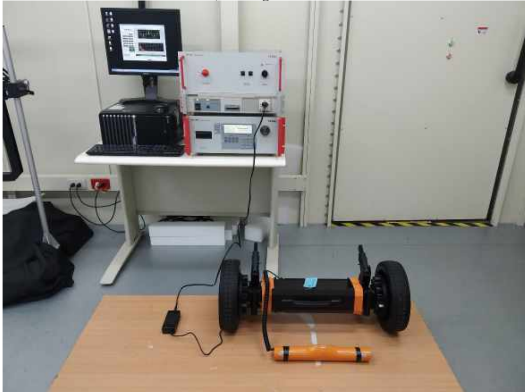
Picture 3: Harmonic Current Emissions, Voltage Fluctuations and Flicker
