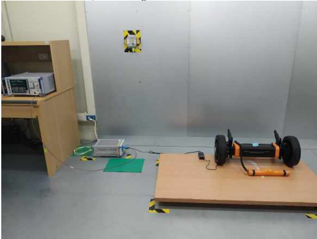
Picture 1: Conducted Emission, Low Voltage AC Mains Port
