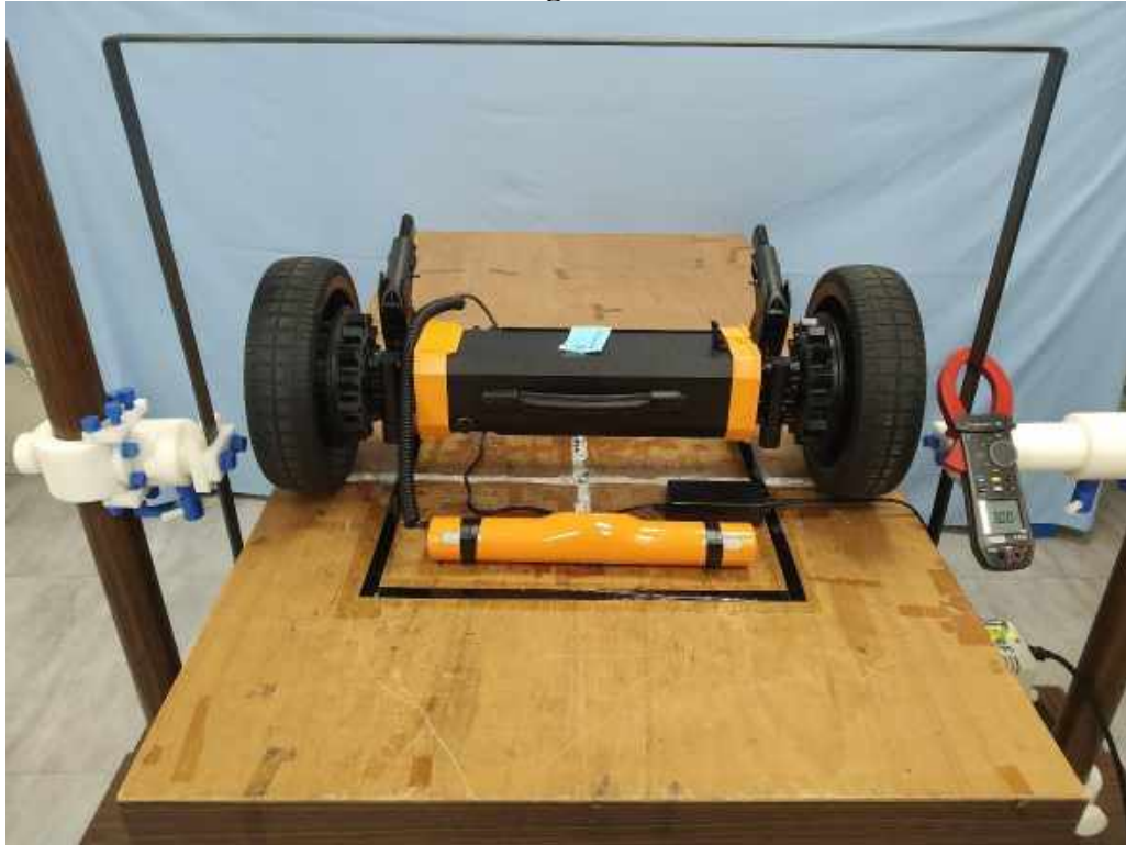
Picture 7: Electrical Fast Transients/Burst
