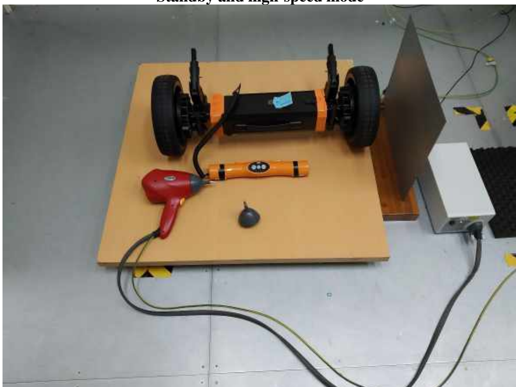
Picture 4: Electrostatic Discharge Standby and high-speed mode
