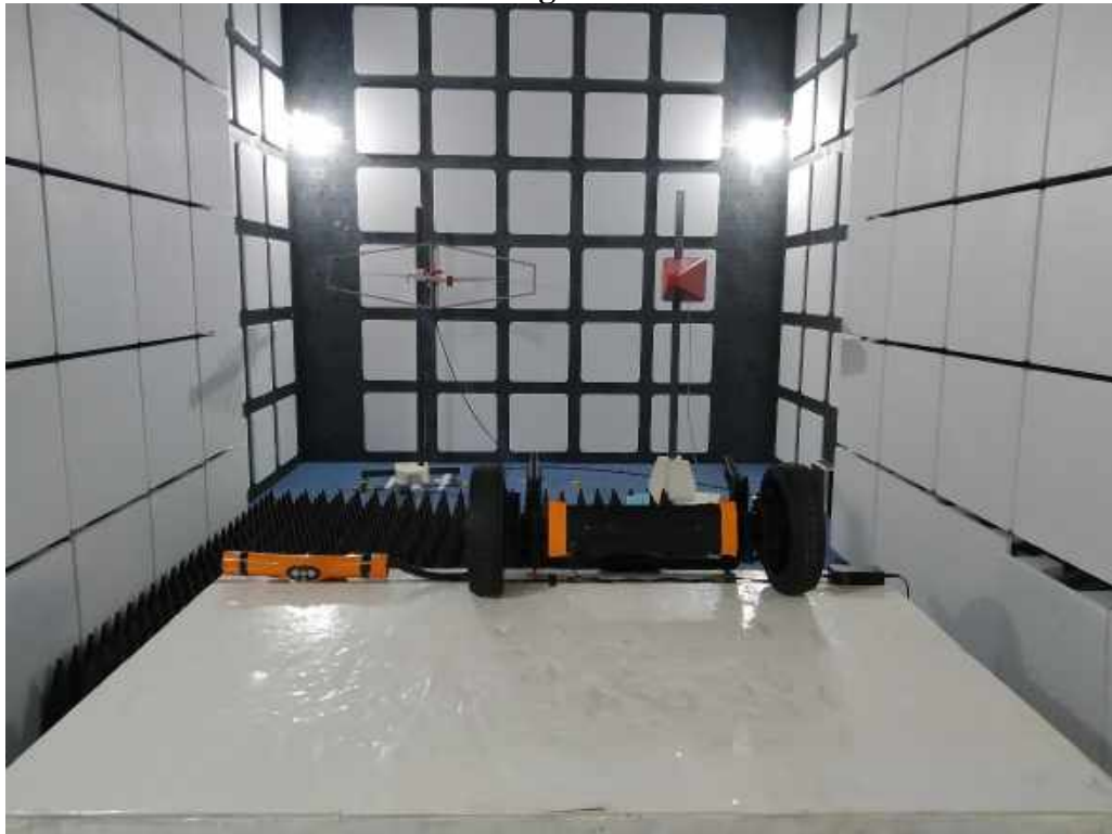
Picture 6: Power Frequency Magnetic Field Standby and high-speed mode
