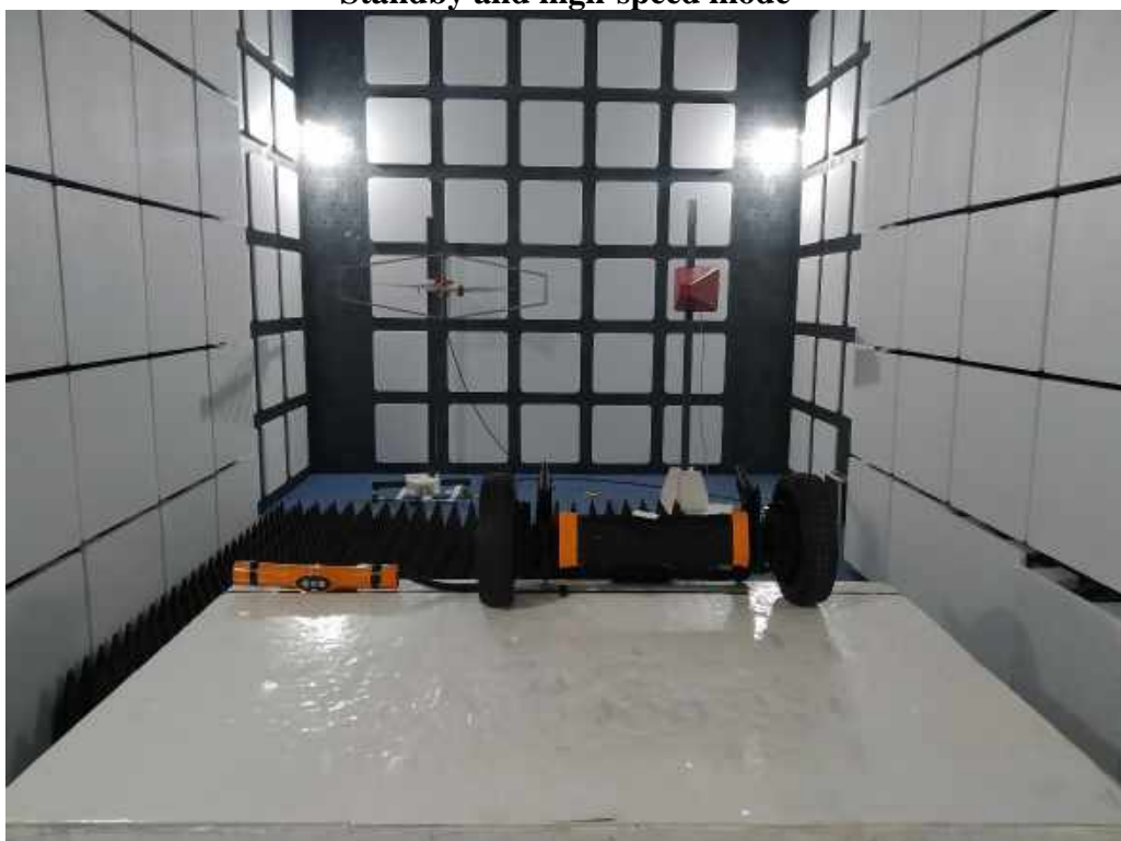
Picture 5: Radio-Frequency Electromagnetic Field Disturbances Standby and high-speed mode
