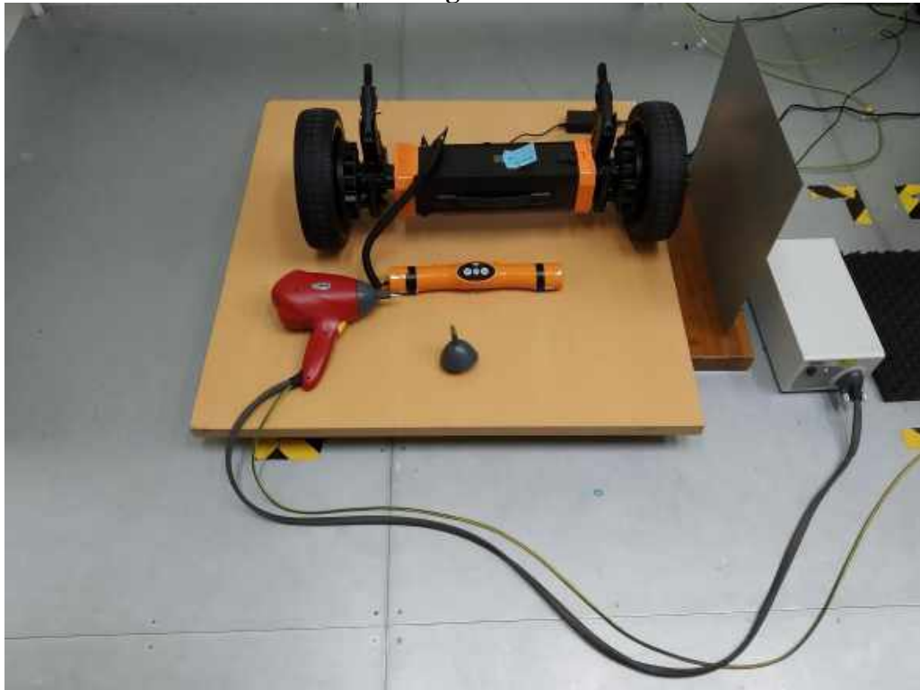
Picture 5: Radio-Frequency Electromagnetic Field Disturbances Standby and high-speed mode
